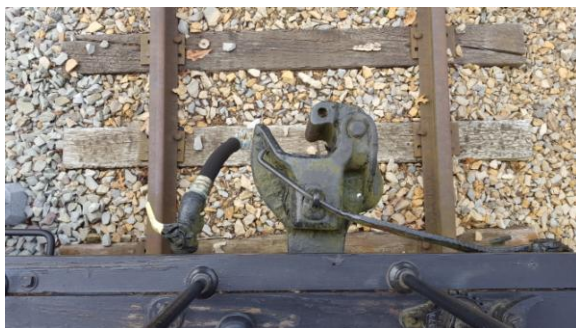
Examples of a knuckle coupler and air hose are on display at the museum’s bobber caboose.
